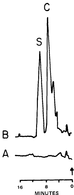
Figure 1 —Elution of fluorescent material from HPLC column after derivatization and extraction of control plasma (A) and plasma from a patient who had taken 100 mg of captopril 1 hr previously (B). Key: C, captopril (I); and S, internal standard (II).
